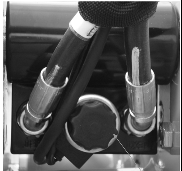
Figure 5-7. Cylinder Valve Removal
