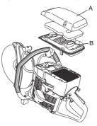
In order to obtain a good filtering effect, the filter must be replaced regularly or cleaned and oiled. A special HUSQVARNA oil has been produced for this purpose.
