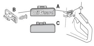
If you want to reactivate the OilGuard system, press the OilGuard plug again. The system is then reactivated, but note that the broken indicator pin cannot be refitted. A broken indicator pin indicates that the OilGuard system has been disconnected. You can purchase a new indicator pin as a spare, but this is only sold in grey which indicates that the OilGuard system has been deactivated since the machine left the factory.
