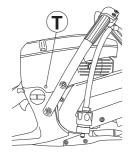
Rec. idle speed: 2700 rpm
