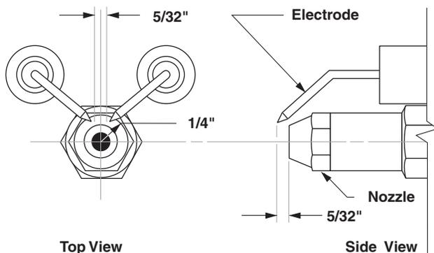
Periodically check wiring connections. If necessary to adjust electrodes, use diagram.
