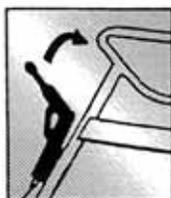
Using lever on handle, lock the one wheel brake (for tighter brake adjustment, turn knob on top of brake lever).
