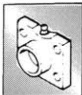
Grease the (2) cutter shaft bearings.
