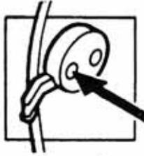
Teeth should be positioned in pockets and tightened to 100 to 110 ft/lbs. torque.
