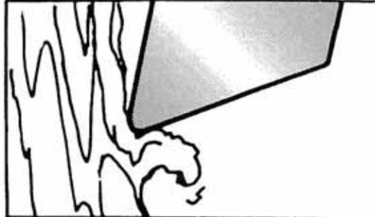
A rounder dull edge creates high cutting pressures, because it must force its way through the material.
