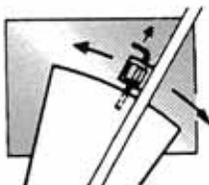
When grinding over 10 inches above or below ground, adjust handle bar for better control and comfort.
