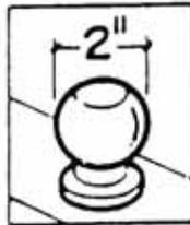
3. **Join grinder to vehicle using 2" ball.**
