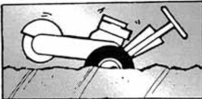
On larger stumps, DO NOT allow stump grinder wheels to drop into hole - fill with chips or change position!
