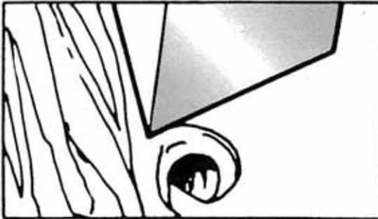
A properly sharpened carbide edge undergoes very little pressure in cutting. A thin, sharp edge slices its way through the material, minimizing resistance.
