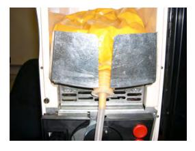
4. Guide the tube through the pump slot from top to bottom.
