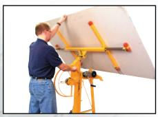
Raise the board off the loader foot bracket by rotating the PANELLIFT® Drywall Lift winch slightly and tilt the board to horizontal.
