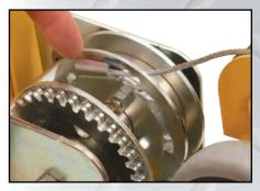
Pull the slack out of the cable to seat the crimped end securely behind the mooring tab as shown.
