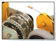
6. Pass the crimped end of the cable over the sheave pocket as shown.
