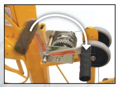
Rotate the winch handle clockwise to take up the slack in the cable around the winch drum.
