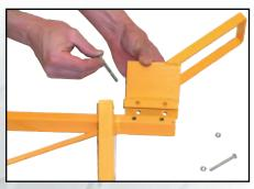
3. Attach the bracket to the loader frame using the 1/4" X 21/4" bolts and lock nuts.
