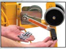
Attach the winch to the loader frame using the 3/8" X 1" bolts with fasteners. NOTE: Install the bolts with flat washers from the top down through the winch and fasten the lock washers and nuts from underneath the winch mount plate.
