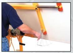
3. When the board is fully raised, swing the cross arm support hooks under the board.
