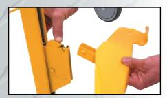
10. Push back on the foot bracket latch, insert bracket, and release latch.
