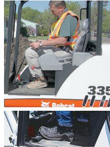
Move steering levers and pedals smoothly. Hydrostatic drive systems are responsive. Excavator will move immediately when controls are activated. Check blade location before moving travel control levers or pedals. Excavator will move in the direction of the blade when steering levers are moved away from the operator.
