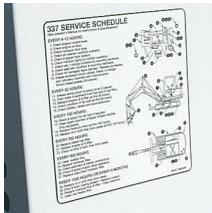
The Service Schedule chart on the machine provides service and maintenance instructions. Check fluid levels, lubricate and grease excavator as required. Check for leaks, broken or damaged parts before operating. **Never smoke when fueling!**
