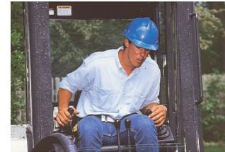
Never operate excavator's controls from the ground. Always sit in the operator's seat when activating the controls.
