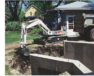
Do not swing loads on a slope. Swing loads low and slowly. Do not travel across or up slopes that are over 15 degrees. Do not travel down or back up slopes that exceed 25 degrees. Keep boom centered.
