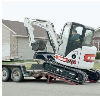
Always drive up the ramp with heavy end uphill (boom, dipper, etc.).
