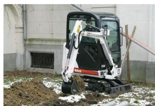
Always look in the direction of travel before moving the excavator or rotating the house swing (slew).
