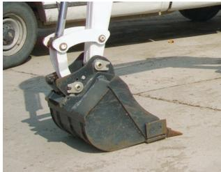
Make sure attachment is securely fastened to excavator. Check that X-Change® system (if equipped) is securely engaged.
